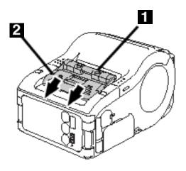
3. Wipe off any dirt on the print head (1) using a soft cloth soaked with some rubbing alcohol.
